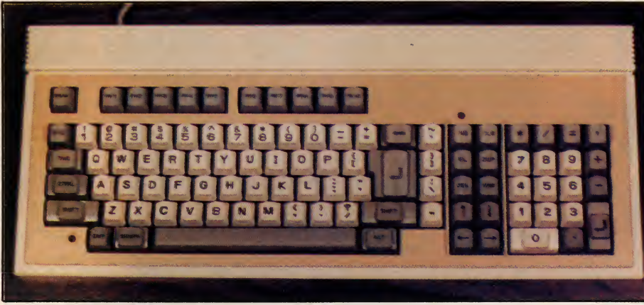
Keyboard has standard alphanumeric portion. Function keys, special keys, and numeric keypad are all separate. Cursor keys are arranged in a reasonably logical way.
